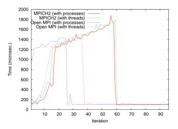
Fig. 9. Concurrent short-long messages test on Linux cluster.
