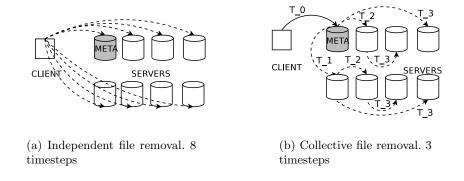
**Fig. 4.** File removal requires deletion of the data file on each server. The independent approach has little room for optimization, requires careful coordination to keep metadata consistent, and needs O(N) timesteps to complete. The collective approach simplifies metadata updates and requires only  $O(\log(N))$  timesteps.
