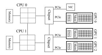
Fig. 1. GPU-accelerated computing system architecture.
